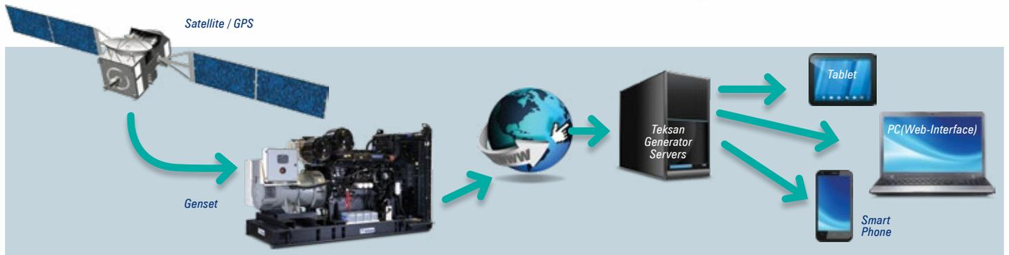
Teksan Remote Monitoring and Management System, supported by GSM and internet technologies, is a highly useful and cost-effective web-based solution that allows remote generator monitoring and intervention when needed. This system, which has the latest technologies, sends the working data of the generator on the field via the control panel to a remote device such as a computer, tablet or smartphone and allows the generator to be managed via this device.
