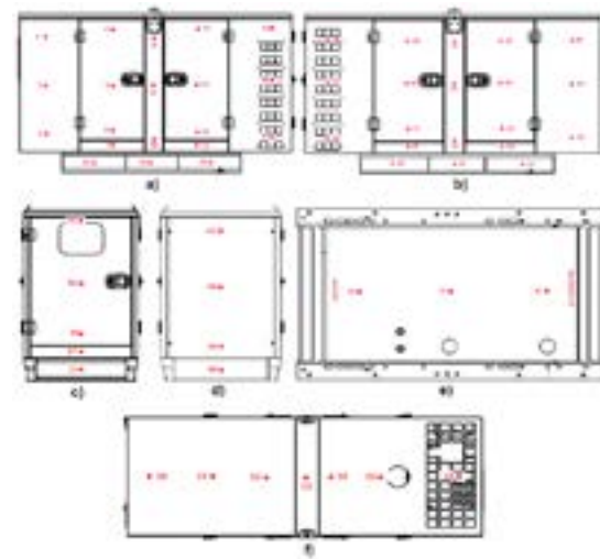
Figure 8: Accelerometer measurement points. a) Left side of the canopy. b) Right side of the canopy. c) Front side of the canopy. d) Back side of the canopy. e) Upper side of the chassis. f) Upper side of the canopy.
